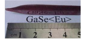
Fig.1. The image of *GaSe* single crystal doped with 0.025 at% *Eu*.
